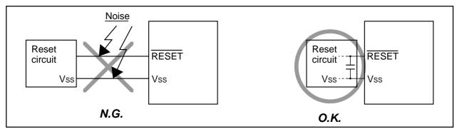
Figure 1.1.2. Wiring for RESET pin
