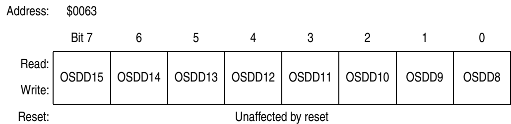
Figure 18-7. OSD Data Register High (OSDDRH)
