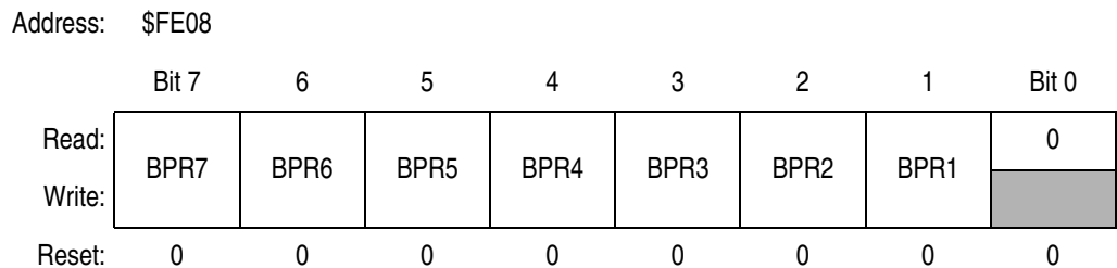
Figure 4-6. 47,616-byte FLASH Block Protect Register (FLBPR)
