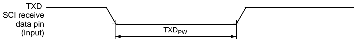
Figure 10-16 TXD Pulse Width
