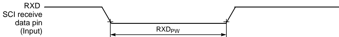
Figure 10-15 RXD Pulse Width
