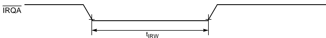
Figure 10-6 External Interrupt Timing (Negative Edge-Sensitive)
