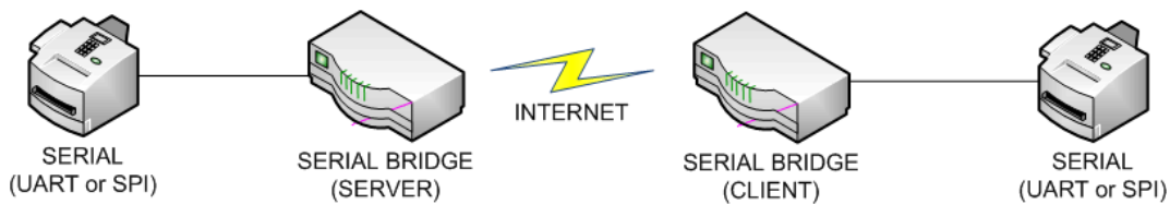
Figure 2. A Serial Device Connected to Another Serial Device Using Client and Server Implementation Using Two Serial Bridges
