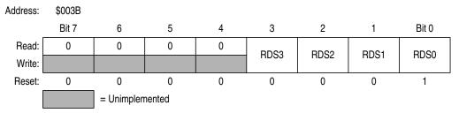
Figure 6-9. PLL Reference Divider Select Register (PMDS)
