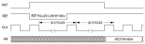
Figure 7-5. Internal Reset Timing
