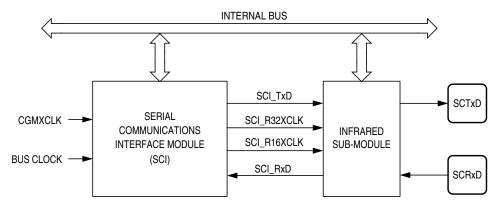
Figure 12-2. IRSCI Block Diagram
