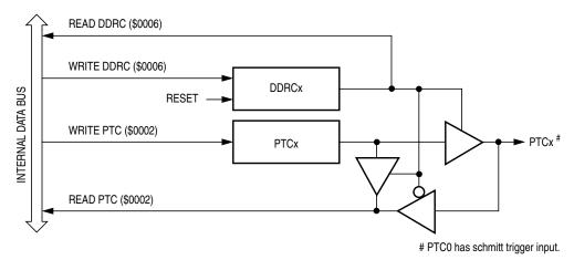
Figure 16-11. Port C I/O Circuit
