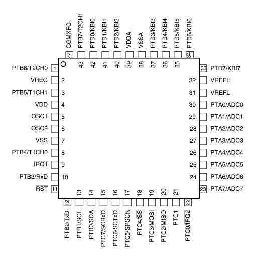
Figure 1-3. 44-Pin QFP Pin Assignments
