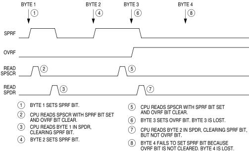
Figure 13-9. Missed Read of Overflow Condition
