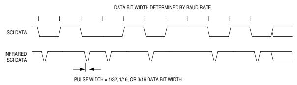
Figure 12-4. Infrared SCI Data Example
