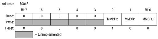
Figure 14-11. MMIIC Frequency Divider Register (MMFDR)
