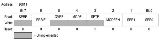
Figure 13-14. SPI Status and Control Register (SPSCR)
