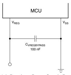
Figure 1-6. Regulator Power Supply Bypassing
