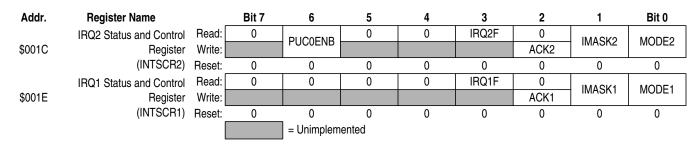
Figure 17-1. External Interrupt I/O Register Summary
