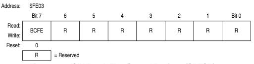
Figure 7-22. SIM Break Flag Control Register (SBFCR)
