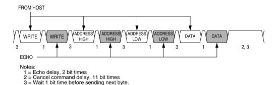
Figure 8-6. Write Transaction
