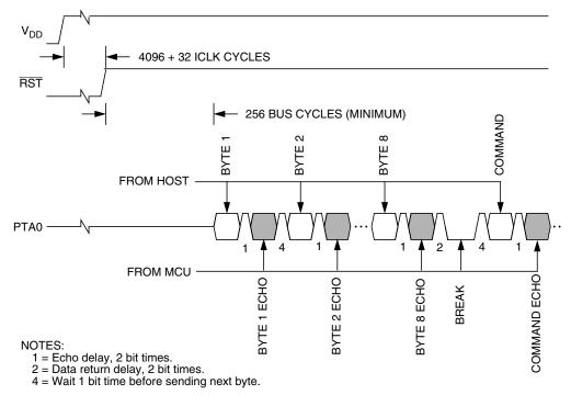
Figure 8-8. Monitor Mode Entry Timing
