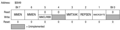
Figure 14-5. MMIIC Control Register 1 (MMCR1)
