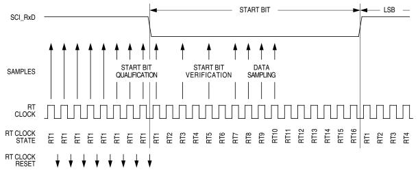
Figure 12-9. Receiver Data Sampling
