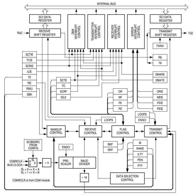
Figure 11-2. SCI Module Block Diagram
