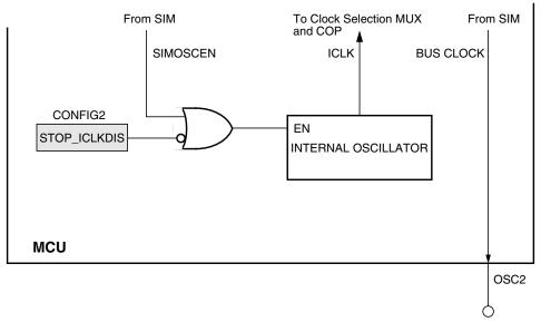
Figure 5-4. Internal Oscillator
