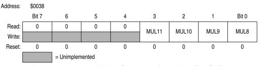
Figure 6-6. PLL Multiplier Select Register High (PMSH)
