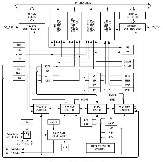
Figure 12-5. SCI Module Block Diagram
