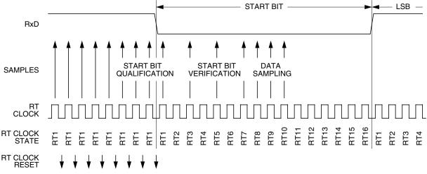
Figure 11-6. Receiver Data Sampling
