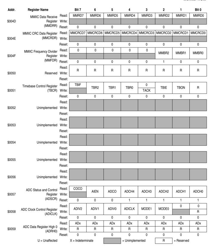
Figure 2-2. Control, Status, and Data Registers (Sheet 7 of 9)
