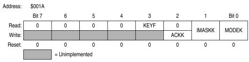
Figure 18-3. Keyboard Status and Control Register (KBSCR)
