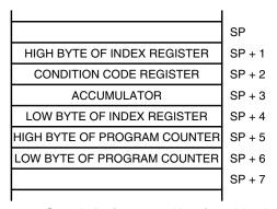
Figure 8-7. Stack Pointer at Monitor Mode Entry
