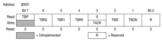
Figure 10-2. Timebase Control Register (TBCR)
