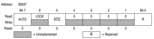
Figure 6-5. PLL Bandwidth Control Register (PBWCR)
