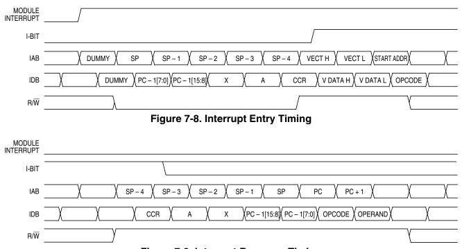
Figure 7-9. Interrupt Recovery Timing
