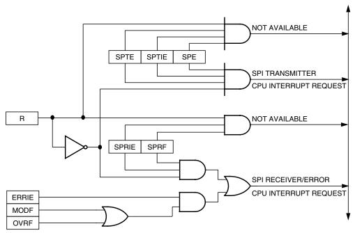
Figure 13-11. SPI Interrupt Request Generation
