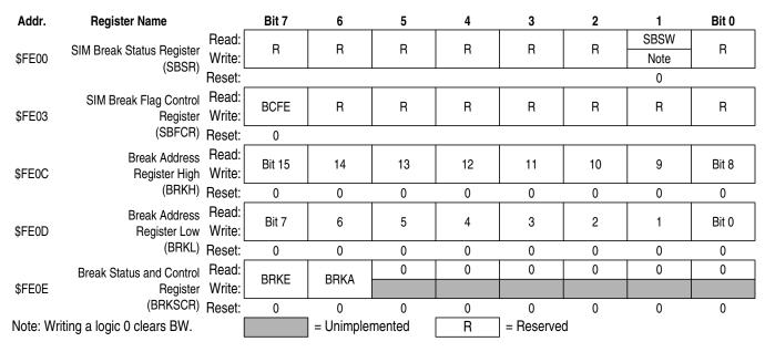
Figure 21-1. Break Module I/O Register Summary
