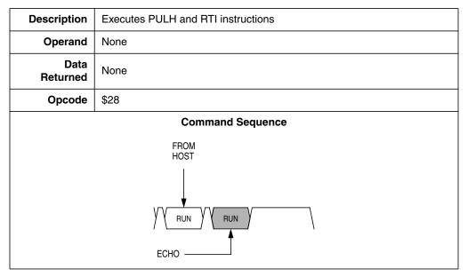
The MCU executes the SWI and PSHH instructions when it enters monitor mode. The RUN command tells the MCU to execute the PULH and RTI instructions. Before sending the RUN command, the host can modify the stacked CPU registers to prepare to run the host program. The READSP command returns the incremented stack pointer value, SP + 1. The high and low bytes of the program counter are at addresses SP + 5 and SP + 6.
