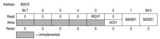
Figure 17-4. IRQ1 Status and Control Register (INTSCR1)
