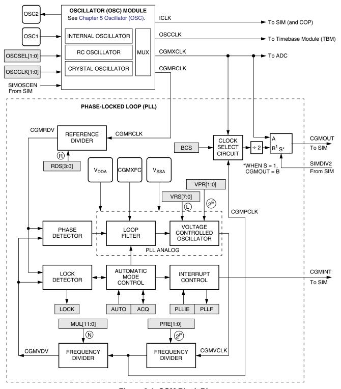
Figure 6-1. CGM Block Diagram
