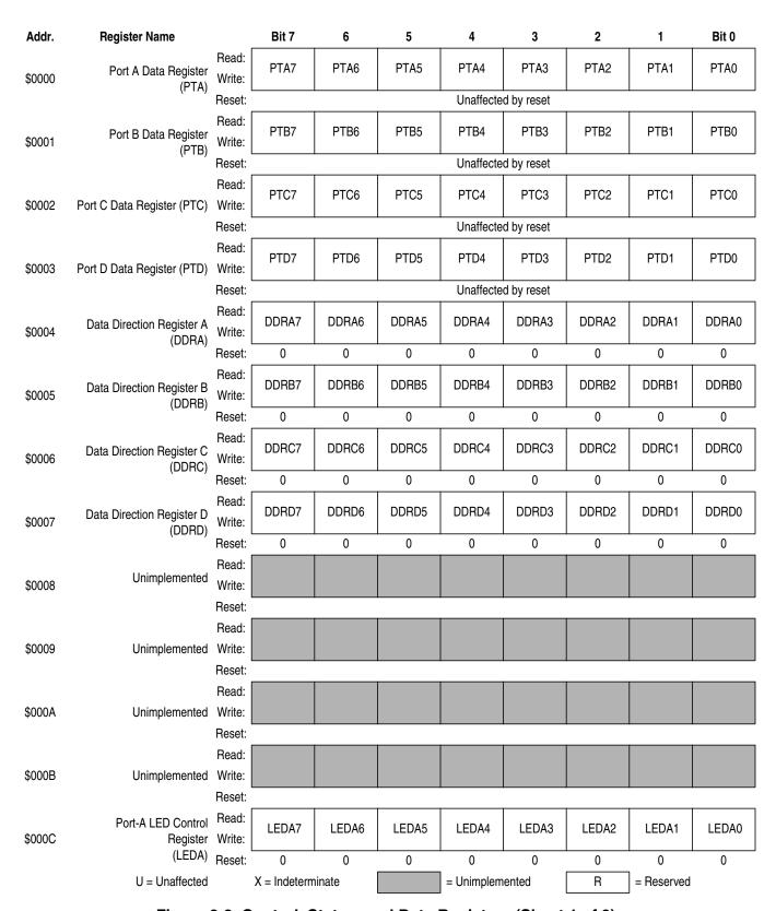
Figure 2-2. Control, Status, and Data Registers (Sheet 1 of 9)
