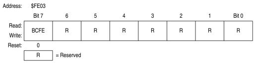
Figure 21-7. SIM Break Flag Control Register (SBFCR)
