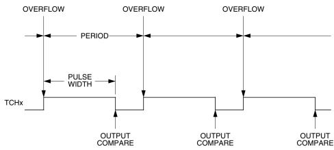
Figure 9-3. PWM Period and Pulse Width
