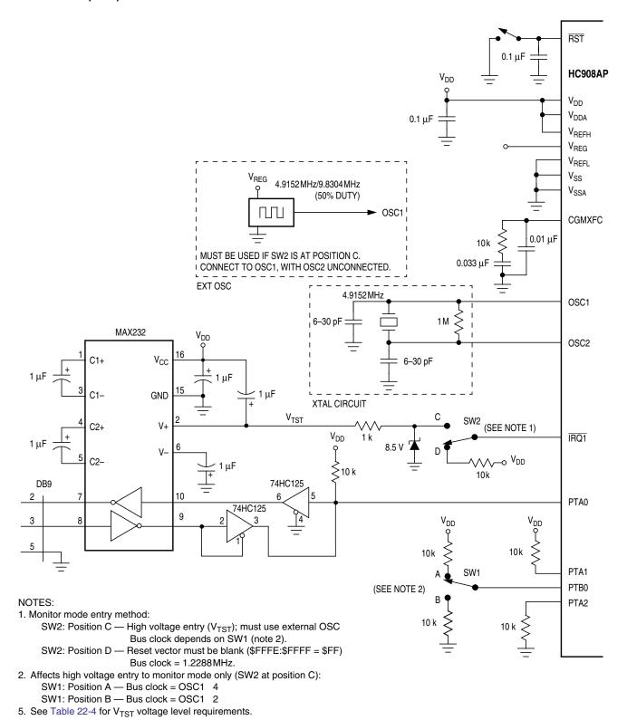
Figure 8-1. Monitor Mode Circuit
