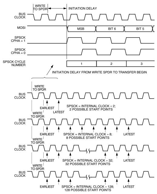
Figure 13-7. Transmission Start Delay (Master)
