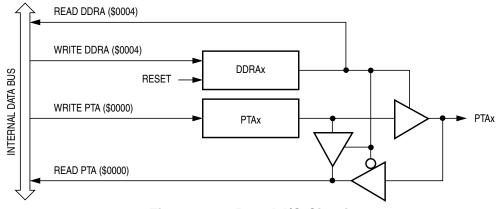
Figure 16-4. Port A I/O Circuit
