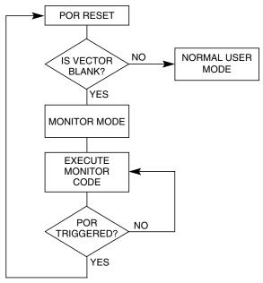
Figure 8-2. Low-Voltage Monitor Mode Entry Flowchart
