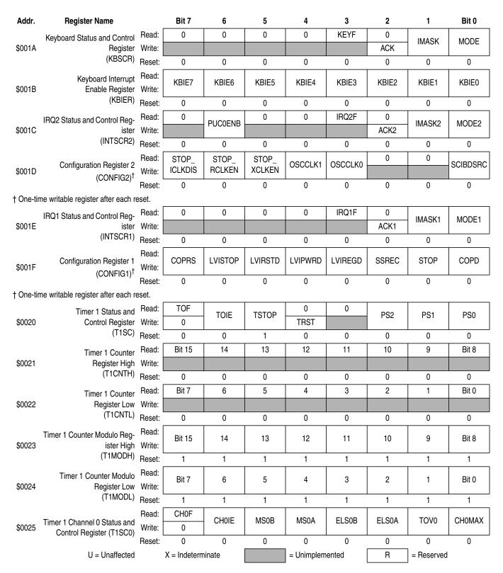
Figure 2-2. Control, Status, and Data Registers (Sheet 3 of 9)
