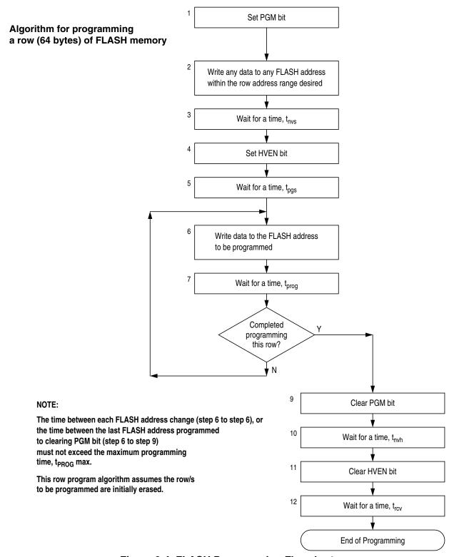
Figure 2-4. FLASH Programming Flowchart
