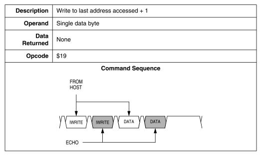
A sequence of IREAD or IWRITE commands can access a block of memory sequentially over the full 64-Kbyte memory map.
