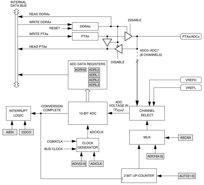
Figure 15-2. ADC Block Diagram
