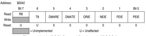
Figure 12-14. IRSCI Control Register 3 (IRSCC3)
