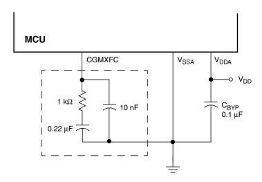
Note: Filter network in box can be replaced with a  $0.47\mu F$  capacitor, but will degrade stability.
