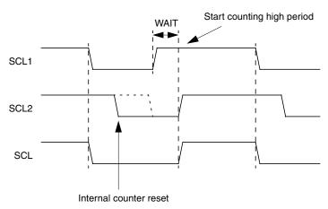
Figure 14-3. Clock Synchronization
