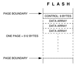
Figure 8-10. EE\_WRITE FLASH Memory Usage
