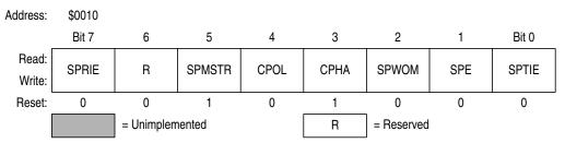
Figure 13-13. SPI Control Register (SPCR)
