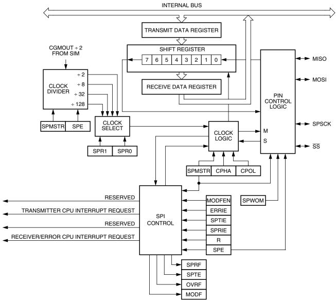
Figure 13-2. SPI Module Block Diagram
