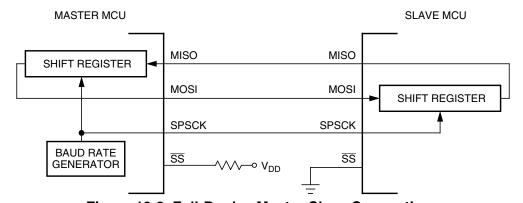
Figure 13-3. Full-Duplex Master-Slave Connections
