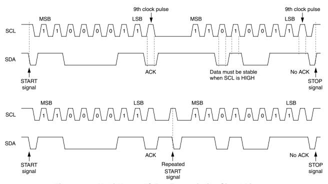
Figure 14-2. Multi-Master IIC Bus Transmission Signal Diagram
