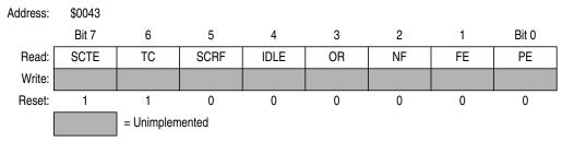
Figure 12-15. IRSCI Status Register 1 (IRSCS1)
