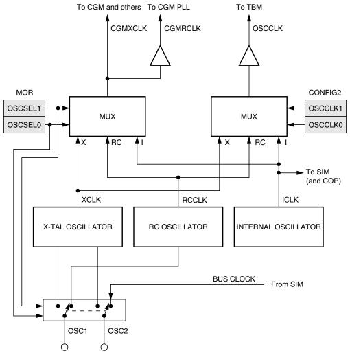
Figure 5-1. Oscillator Module Block Diagram
