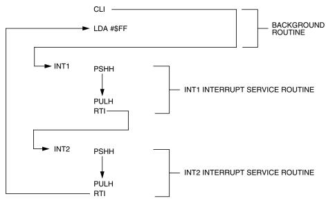
Figure 7-11. Interrupt Recognition Example
