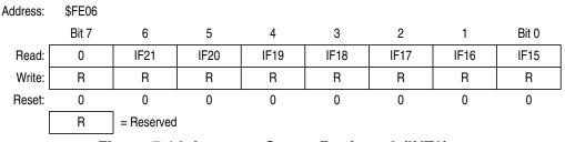
Figure 7-14. Interrupt Status Register 3 (INT3)
