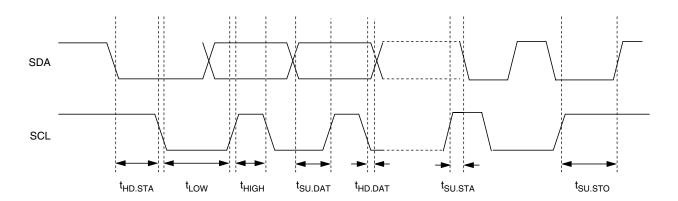
Figure 22-2. MMIIC Signal Timings
