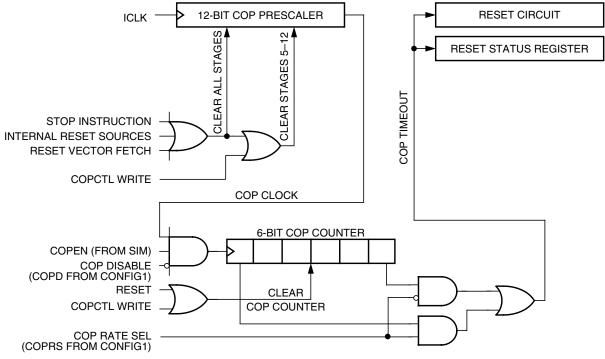
Figure 19-1. COP Block Diagram
