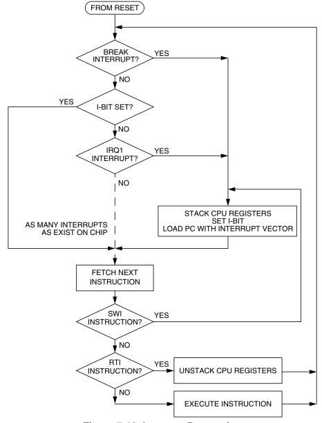
Figure 7-10. Interrupt Processing
