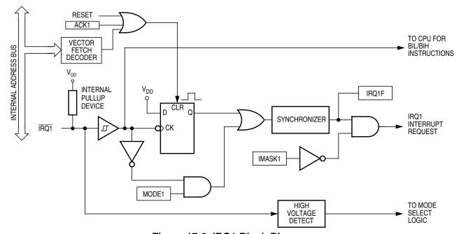
Figure 17-2. IRQ1 Block Diagram
