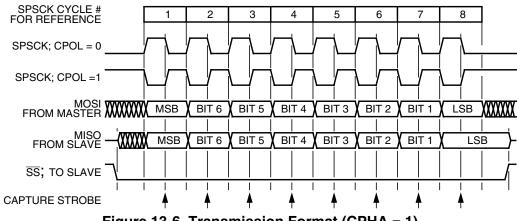
Figure 13-6. Transmission Format (CPHA = 1)
