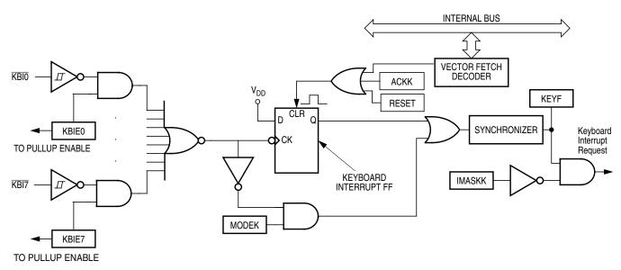
Figure 18-2. Keyboard Interrupt Block Diagram
