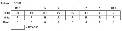
Figure 7-12. Interrupt Status Register 1 (INT1)
