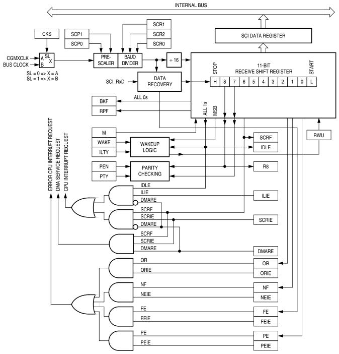
Figure 12-8. SCI Receiver Block Diagram
