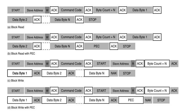
Figure 14-19. Block Read/Write
