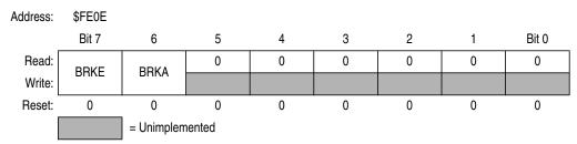
Figure 21-3. Break Status and Control Register (BRKSCR)
