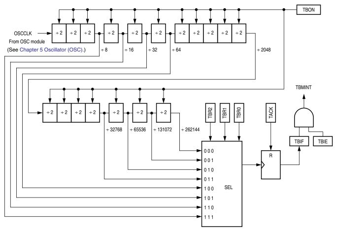
Figure 10-1. Timebase Block Diagram
