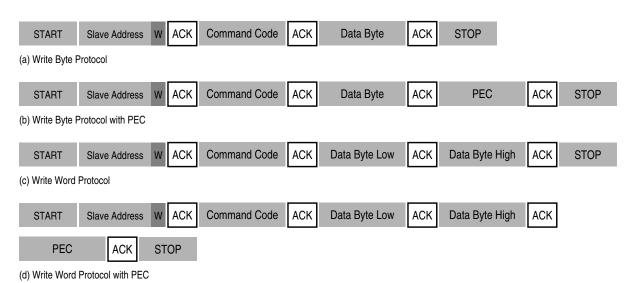
Figure 14-16. Write Byte/Word
