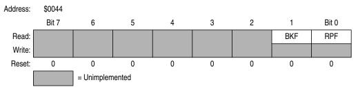
Figure 12-17. IRSCI Status Register 2 (IRSCS2)
