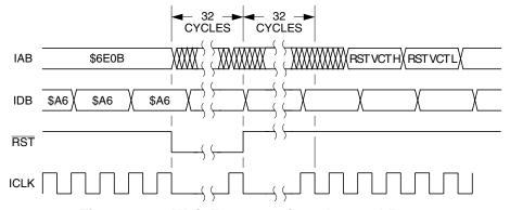
Figure 7-17. Wait Recovery from Internal Reset
