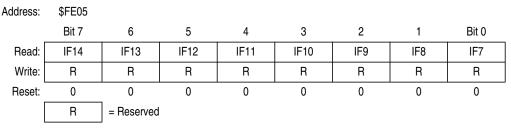
Figure 7-13. Interrupt Status Register 2 (INT2)
