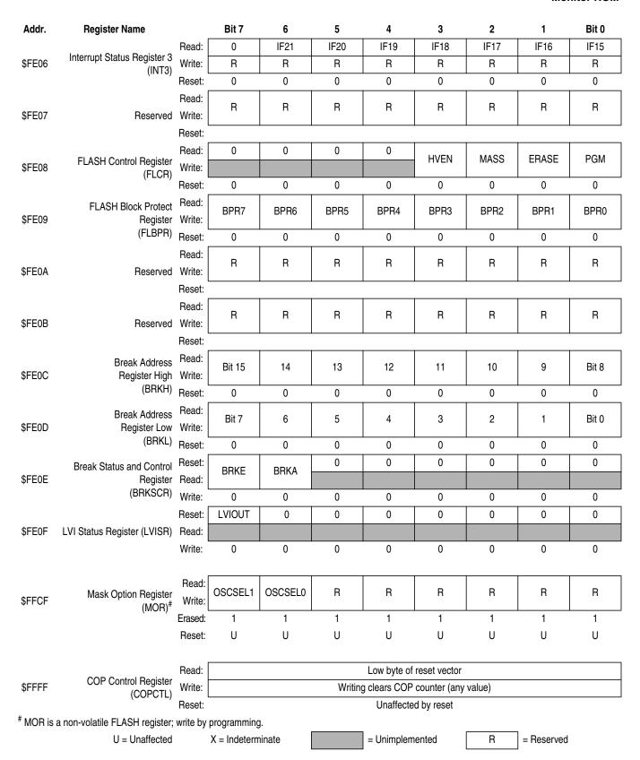
Figure 2-2. Control, Status, and Data Registers (Sheet 9 of 9)
