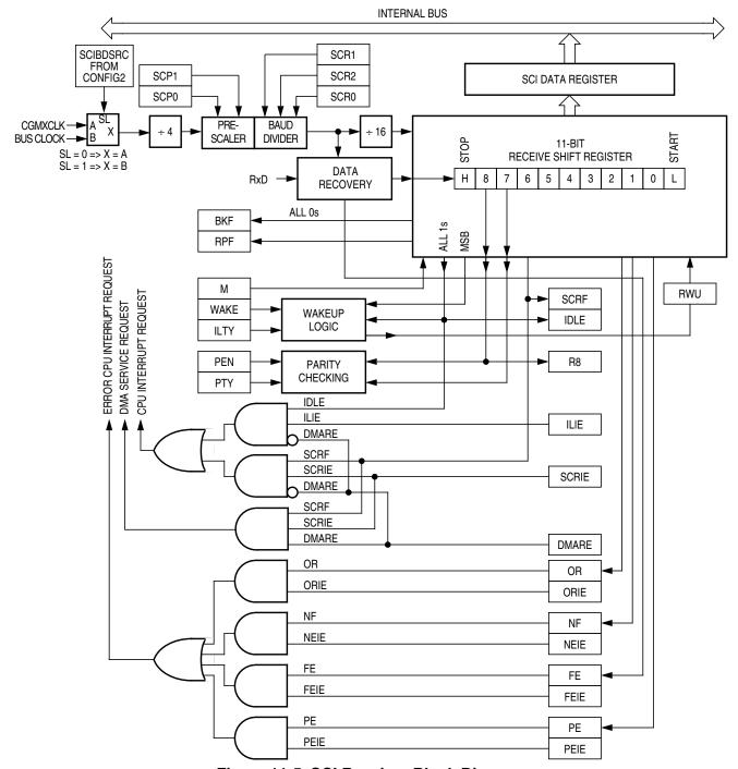
Figure 11-5. SCI Receiver Block Diagram
