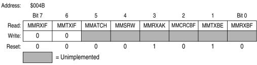
Figure 14-7. MMIIC Status Register (MMSR)
