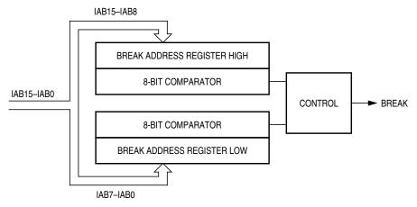
Figure 21-2. Break Module Block Diagram
