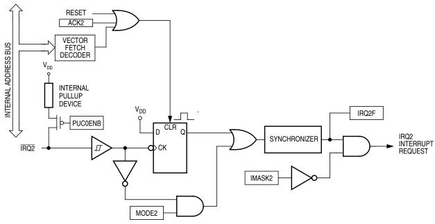
Figure 17-3. IRQ2 Block Diagram
