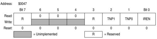
Figure 12-20. IRSCI Infrared Control Register (IRSCIRCR)
