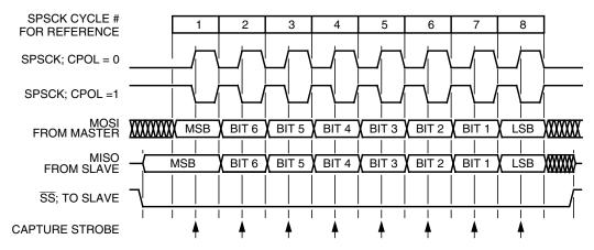
Figure 13-4. Transmission Format (CPHA = 0)
