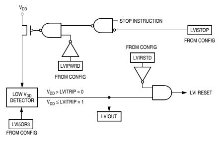
Figure 10-1. LVI Module Block Diagram
