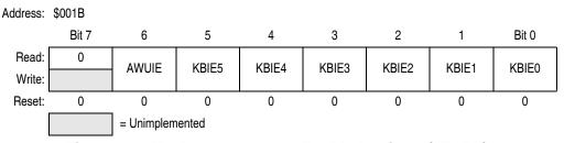
Figure 9-4. Keyboard Interrupt Enable Register (KBIER)
