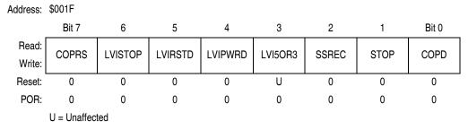
Figure 5-2. Configuration Register 1 (CONFIG1)
