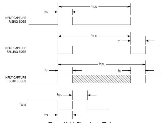
Figure 16-11. Timer Input Timing
