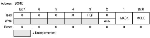
Figure 8-3. IRQ Status and Control Register (INTSCR)
