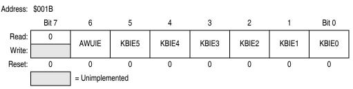
Figure 4-4. Keyboard Interrupt Enable Register (KBIER)
