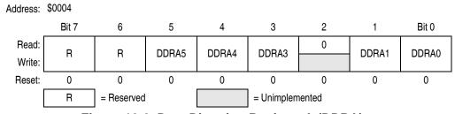
Figure 12-2. Data Direction Register A (DDRA)
