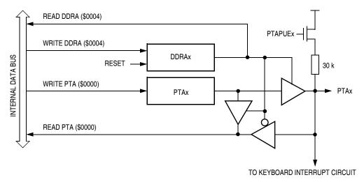
Figure 12-3. Port A I/O Circuit
