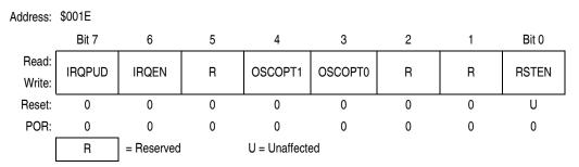
Figure 5-1. Configuration Register 2 (CONFIG2)
