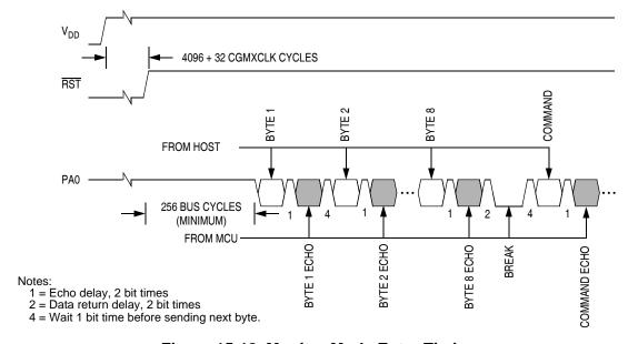
Figure 15-18. Monitor Mode Entry Timing
