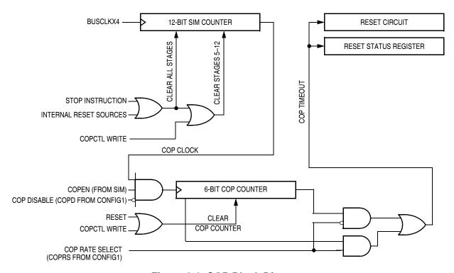
Figure 6-1. COP Block Diagram
