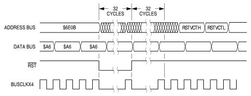
Figure 13-16. Wait Recovery from Internal Reset
