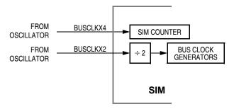
Figure 13-2. SIM Clock Signals
