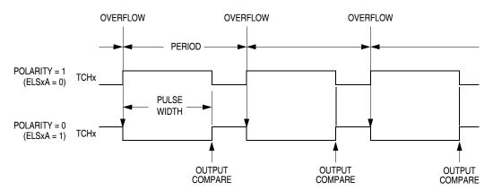
Figure 14-3. PWM Period and Pulse Width
