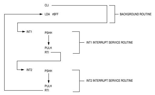
Figure 13-10. Interrupt Recognition Example
