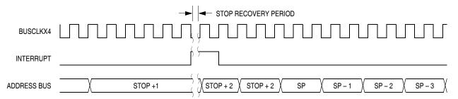
Figure 13-18. Stop Mode Recovery from Interrupt
