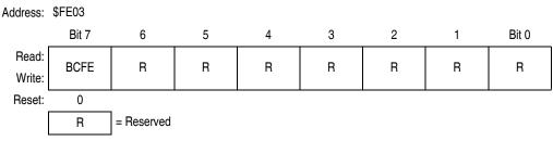
Figure 15-8. Break Flag Control Register (BFCR)
