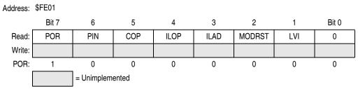
Figure 13-19. SIM Reset Status Register (SRSR)
