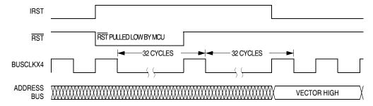
Figure 13-4. Internal Reset Timing
