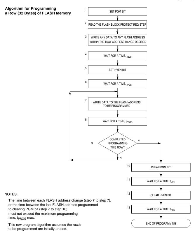
Figure 2-4. FLASH Programming Flowchart
