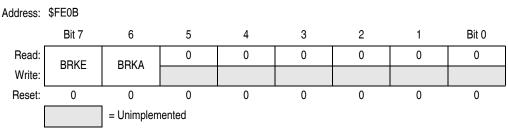
Figure 15-3. Break Status and Control Register (BRKSCR)
