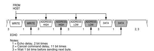
Figure 15-16. Write Transaction
