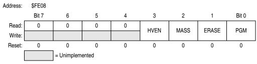
Figure 2-3. FLASH Control Register (FLCR)
