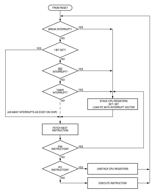
Figure 13-7. Interrupt Processing
