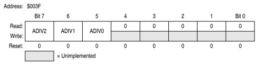
Figure 3-5. ADC Input Clock Register (ADICLK)
