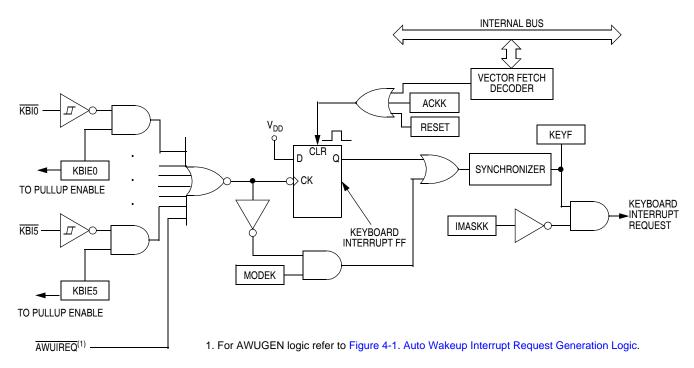
Figure 9-2. Keyboard Interrupt Block Diagram
