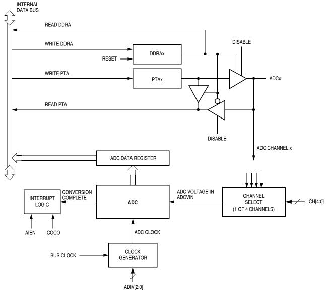
Figure 3-2. ADC Block Diagram
