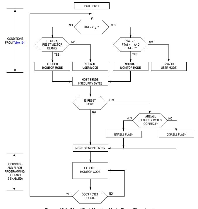
Figure 15-9. Simplified Monitor Mode Entry Flowchart
