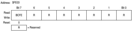
Figure 13-20. Break Flag Control Register (BFCR)
