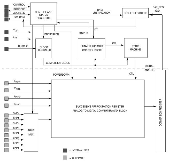
Figure 14-2. ATD Block Diagram
