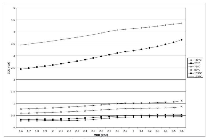
Figure A-8. Typical Stop 2 I<sub>DD</sub>
