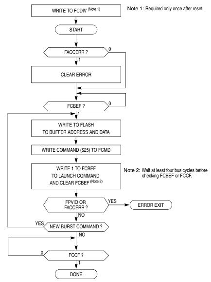
Figure 4-3. FLASH Burst Program Flowchart
