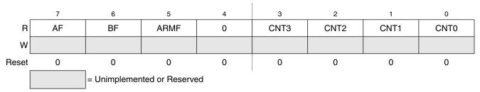
Figure 15-9. Debug Status Register (DBGS)
