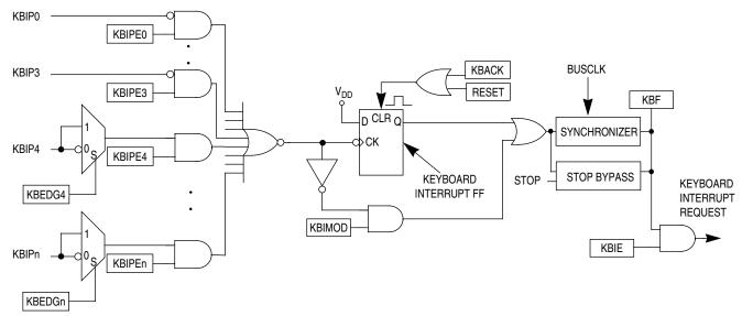
Figure 7-3. KBI Block Diagram
