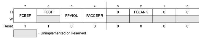
Figure 4-9. FLASH Status Register (FSTAT)
