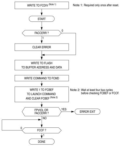
Figure 4-2. FLASH Program and Erase Flowchart
