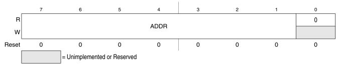
Figure 13-3. IIC Address Register (IICA)
