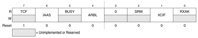
Figure 13-6. IIC Status Register (IICS)
