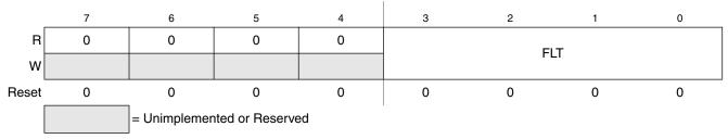
Figure 9-10. ICG Upper Filter Register (ICGFLTU)
