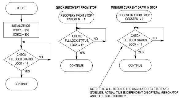
Figure 9-14. ICG Initialization for FEE in Example #1
