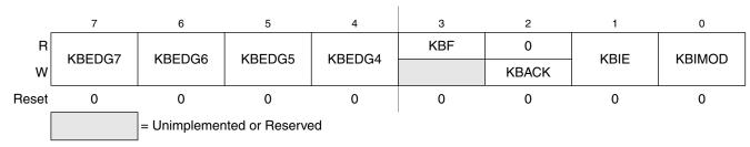
Figure 7-4. KBI Status and Control Register (KBISC)
