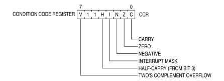
Figure 8-2. Condition Code Register
