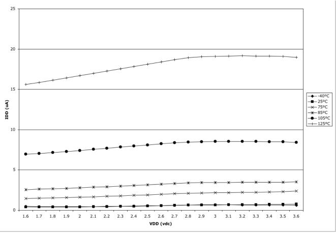
Figure A-9. Typical Stop3 I<sub>DD</sub>
