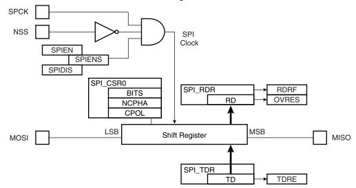
Figure 28-9. Slave Mode Functional Block Diagram
