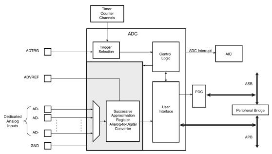
Figure 33-1. Analog-to-Digital Converter Block Diagram
