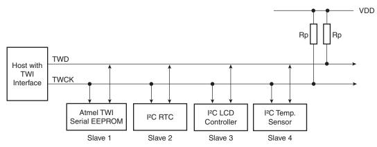
Figure 29-5. Master Mode Typical Application Block Diagram
