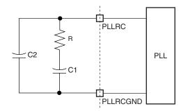
Values of R, C1 and C2 to be connected to the PLLRC pin must be calculated as a function of the PLL input frequency, the PLL output frequency and the phase margin. A trade off has to be found between output signal overshoot and startup time. See the product electrical PLL characteristics section.
