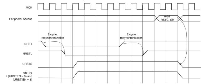
Figure 13-7. Reset Controller Status and Interrupt
