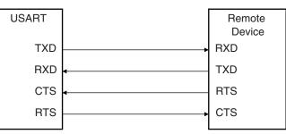
Figure 30-27. Connection with a Remote Device for Hardware Handshaking
