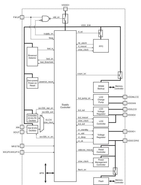
Figure 17-1. Supply Controller Block Diagram
