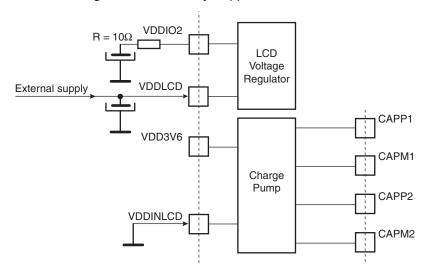
Figure 5-4. The LCD Regulator is Externally Supplied
