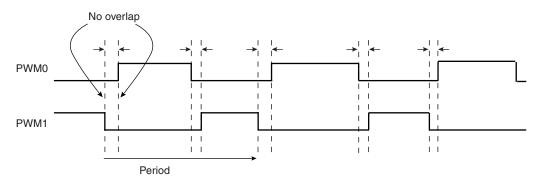
Note: 1. See Figure 32-5 on page 459 for a detailed description of center aligned waveforms. When center aligned, the internal channel counter increases up to CPRD and decreases down to 0. This ends the period.
