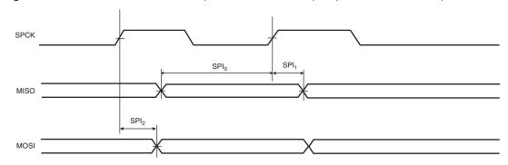
Figure 35-13. SPI Master Mode with (CPOL= NCPHA = 0) or (CPOL= NCPHA= 1)
