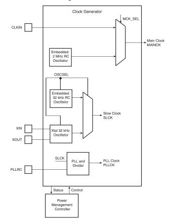
Figure 9-2. Clock Generator Block Diagram
