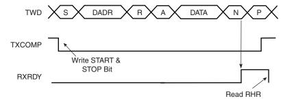
Figure 29-10. Master Read with Multiple Data Bytes
