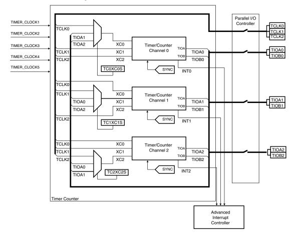
Figure 31-1. Timer Counter Block Diagram
