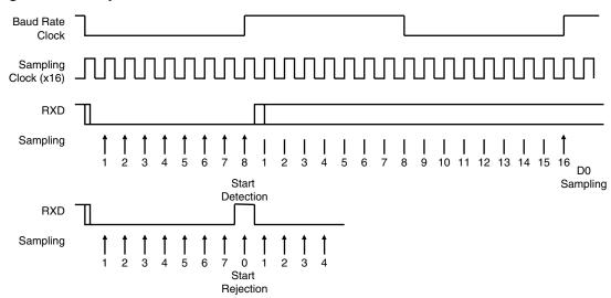
Figure 30-13. Asynchronous Character Reception
