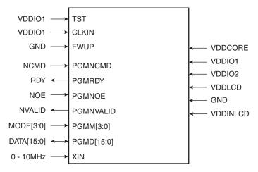
Figure 20-1. Parallel Programming Interface
