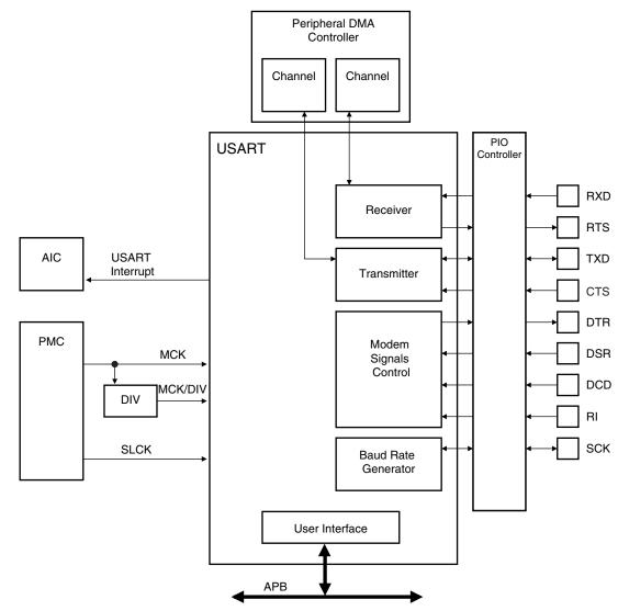
Figure 30-1. USART Block Diagram
