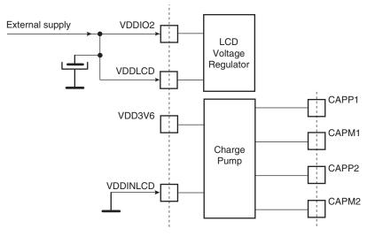
Please note that in this topology, switching time enhancement buffers are not available. (Refer Section 10.13 "Segment LCD Controller".)
