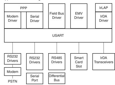
Figure 30-2. Application Block Diagram
