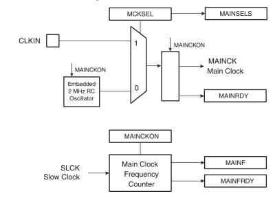
Figure 24-3. Main Clock Block Diagram
