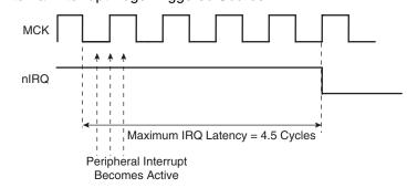
Figure 23-8. Internal Interrupt Edge Triggered Source
