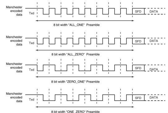
Figure 30-9. Preamble Patterns, Default Polarity Assumed
