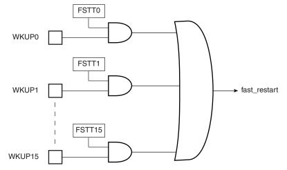
Each wake-up input pin can be enabled to generate a Fast Startup event by writing at 1 the corresponding bit in the Fast Startup Mode Register SUPC\_FSMR. Only a low level on the enabled wake-up input pins generates a Fast Startup.
