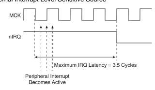
Figure 23-9. Internal Interrupt Level Sensitive Source
