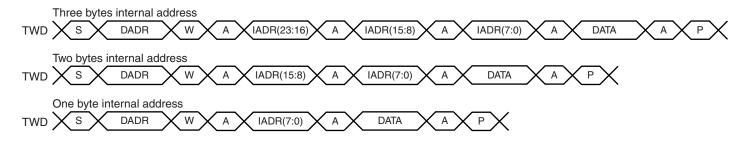
Figure 29-12. Master Read with One, Two or Three Bytes Internal Address and One Data Byte
