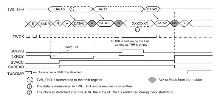
Figure 29-27. Clock Synchronization in Read Mode
