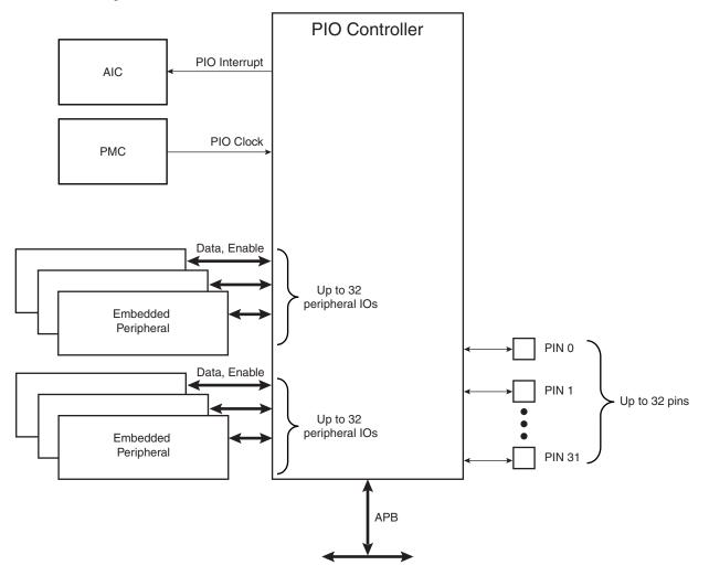
Figure 27-2. Application Block Diagram
