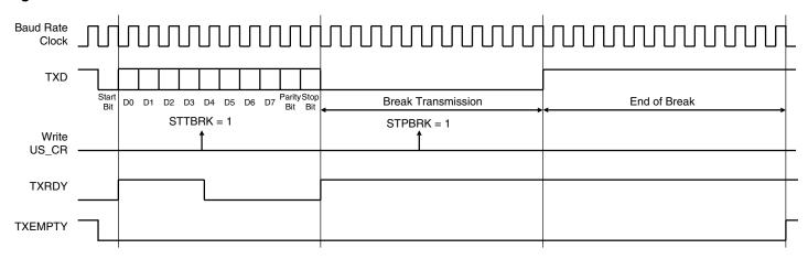
Figure 30-26. Break Transmission
