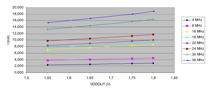
**Figure 35-10.** High-range Frequencies, Active Mode Consumption @25°C (Peripheral Clocks Off - PLL On - RC Off - VDD0I1 = 3V)
