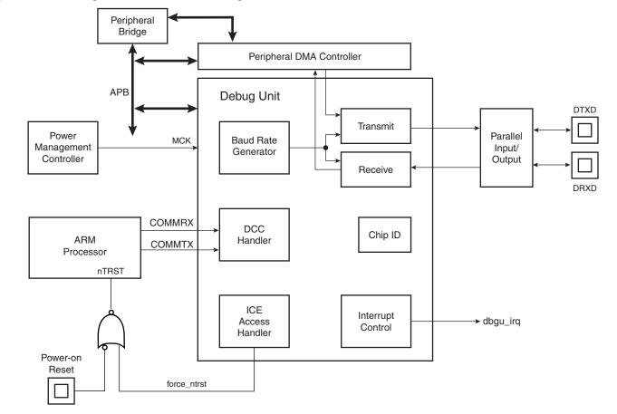
Figure 26-1. Debug Unit Functional Block Diagram
