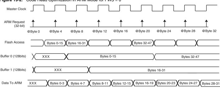
Figure 19-2. Code Read Optimization in ARM Mode for FWS = 0
