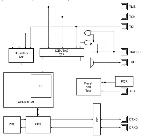
Figure 12-1. Debug and Test Block Diagram
