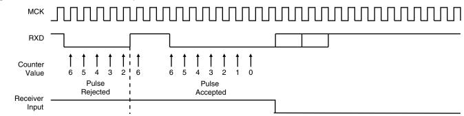
Figure 30-35. IrDA Demodulator Operations
