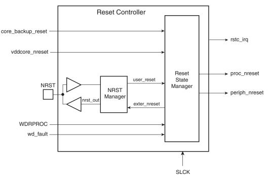
Figure 13-1. Reset Controller Block Diagram
