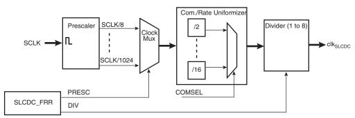
Figure 34-2. Clock Generation Block Diagram
