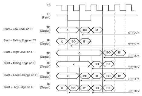
Figure 32-11. Receive Pulse/Edge Start Modes
