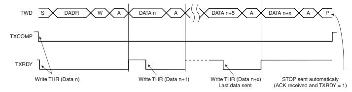
Figure 29-7. Master Write with One Byte Internal Address and Multiple Data Bytes
