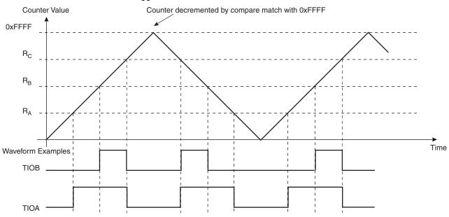
Figure 33-12. WAVSEL = 01 With Trigger
