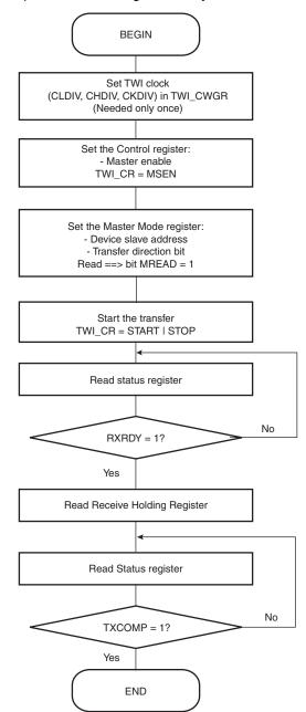
Figure 29-17. TWI Read Operation with Single Data Byte and Internal Address
