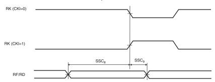
Figure 37-13. SSC Receiver, RK in input and RF in output
