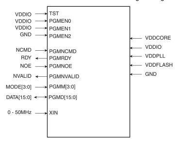
Figure 20-2. AT91SAM7S32/16 Parallel Programming Interface
