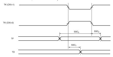
Figure 37-12. SSC Receiver RK and RF in input
