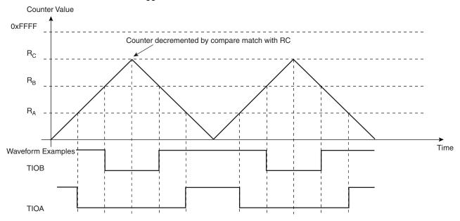
Figure 33-14. WAVSEL = 11 With Trigger
