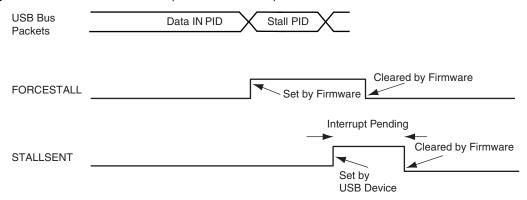
Figure 35-13. Stall Handshake (Data OUT Transfer)
