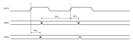
Figure 37-5. SPI Master mode with (CPOL=0 and NCPHA=1) or (CPOL=1 and NCPHA=0)
