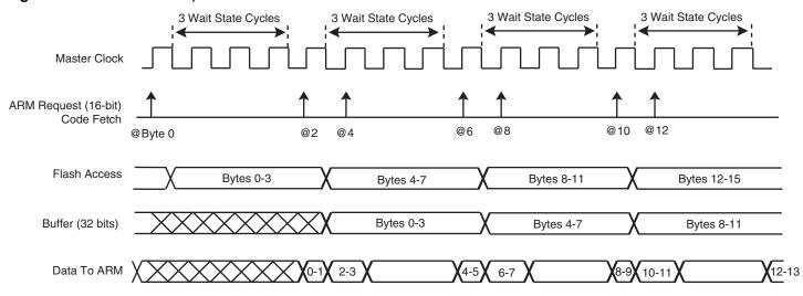
Note: When FWS is equal to 2 or 3, in case of sequential reads, the first access takes FWS cycles, the second access one cycle, the third access FWS cycles, the fourth access one cycle, etc.
