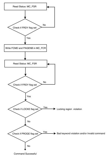
In order to guarantee valid operations on the Flash memory, the field Flash Microsecond Cycle Number (FMCN) in the Flash Mode Register MC\_FMR must be correctly programmed (see "MC Flash Mode Register" on page 116).
