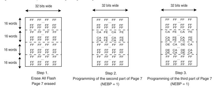
The Partial Programming mode works only with 32-bit (or higher) boundaries. It cannot be used with boundaries lower than 32 bits (8 or 16-bit for example).
