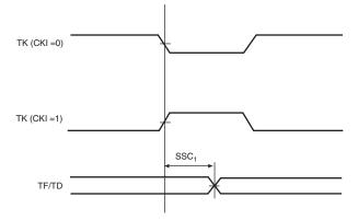
Figure 37-10. SSC Transmitter, TK in output and TF in input
