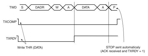
Figure 29-6. Master Write with Multiple Data Byte
