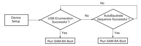
Figure 21-2. Boot Program Algorithm Flow Diagram without USB
