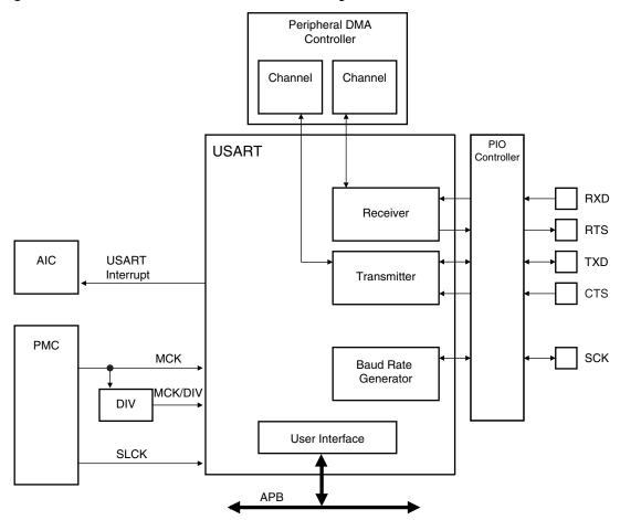
Figure 31-2. AT91SAM7S32/16 USART Block Diagram
