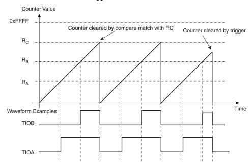
Figure 33-10. WAVSEL = 10 With Trigger
