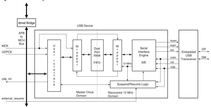
Access to the UDP is via the APB bus interface. Read and write to the data FIFO are done by reading and writing 8-bit values to APB registers.
