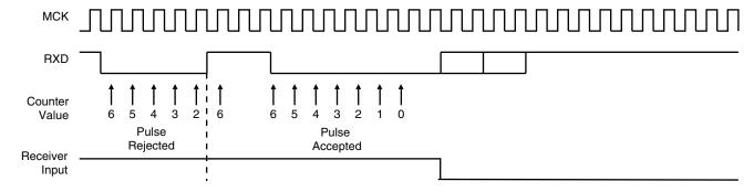
As the IrDA mode uses the same logic as the ISO7816, note that the FI\_DI\_RATIO field in US\_FIDI must be set to a value higher than 0 in order to assure IrDA communications operate correctly.
