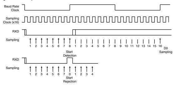
Figure 31-11. Asynchronous Character Reception
