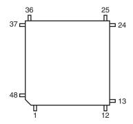
Figure 4-4. 48-pad QFN Package (Top View)
