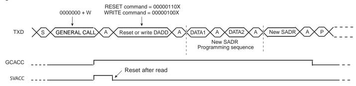
Note: This method allows the user to create an own programming sequence by choosing the programming bytes and the number of them. The programming sequence has to be provided to the master.
