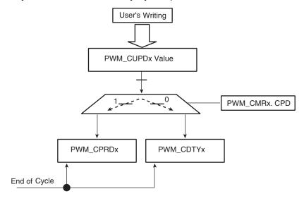
To prevent overwriting the PWM\_CUPDx by software, the user can use status events in order to synchronize his software. Two methods are possible. In both, the user must enable the dedicated interrupt in PWM\_IER at PWM Controller level.
