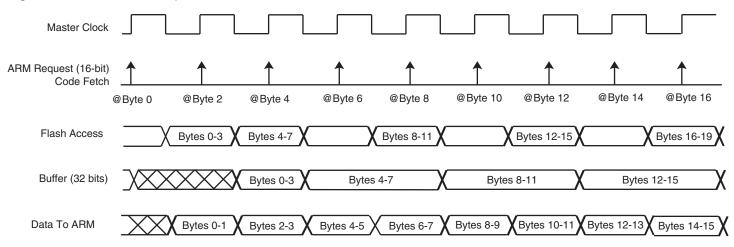
Note: When FWS is equal to 0, all accesses are performed in a single-cycle access.
