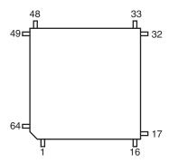
Figure 4-2. 64-pad QFN Package (Top View)
