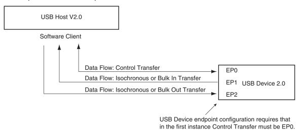
The Control Transfer endpoint EP0 is always used when a USB device is first configured (USB v. 2.0 specifications).
