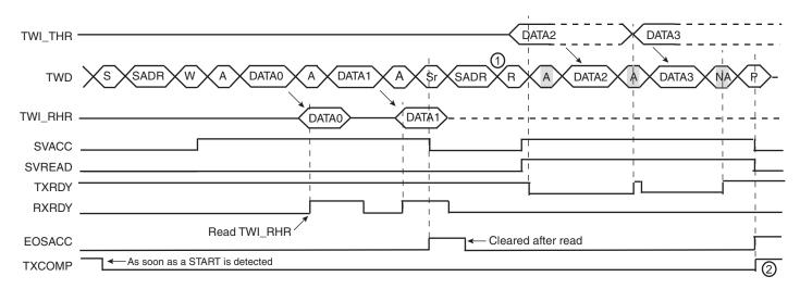
Notes: 1. In this case, if TWI\_THR has not been written at the end of the read command, the clock is automatically stretched before the ACK.
