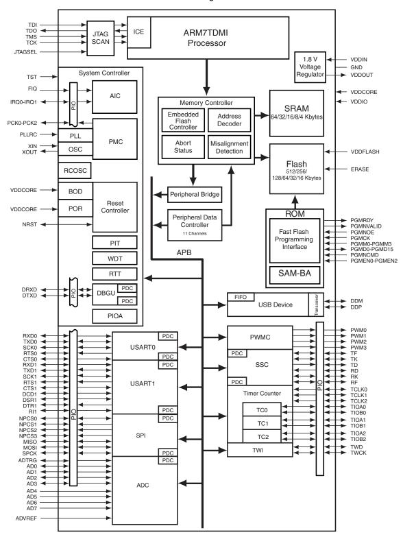
Figure 2-2. AT91SAM7S32/16 Block Diagram
