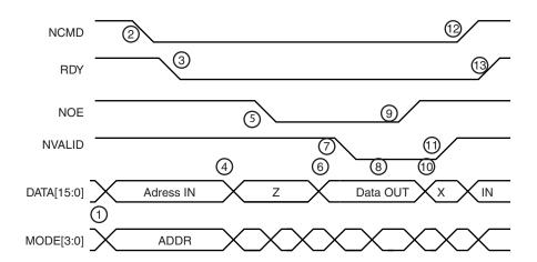
Figure 20-6. AT91SAM7S32/16 Parallel Programming Timing, Read Sequence
