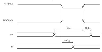
Figure 37-15. SSC Receiver, RK in output and RF in input
