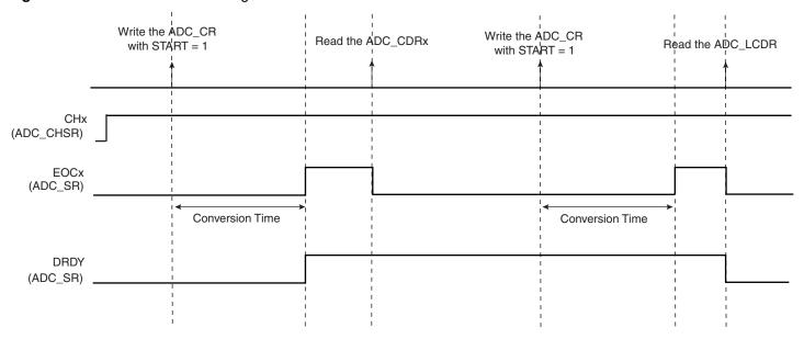
If the ADC\_CDR is not read before further incoming data is converted, the corresponding Overrun Error (OVRE) flag is set in the Status Register (ADC\_SR).
