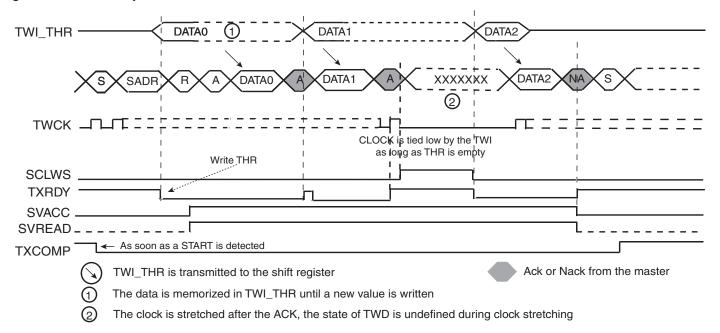
Notes: 1. TXRDY is reset when data has been written in the TWI\_TH to the shift register and set when this data has been acknowledged or non acknowledged.
