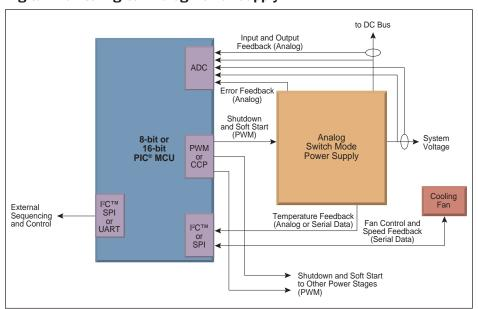
soft-start profiles and current limits can be programmed to suit the application. The output voltage can be fine-tuned to provide coordination between multiple power supplies in a system. Depending on the system I/O requirements, 8-bit solutions in the PIC12, PIC16 or PIC18 device families can provide the ideal solution. In larger systems, the 16-bit PIC24 device family can provide more communication peripherals.
