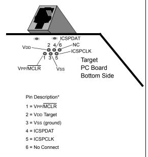
Another connector often found in use with the PICkit<sup>™</sup> programmers is a standard 6-pin header with 0.1 inch spacing. Refer to Figure 28-3.
