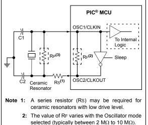
3: An additional parallel feedback resistor (RP) may be required for proper ceramic resonator operation.
