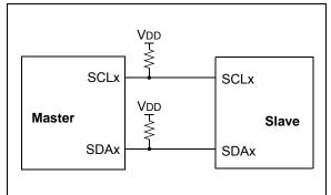
The Acknowledge bit  $(\overline{ACK})$  is an active-low signal, which holds the SDAx line low to indicate to the transmitter that the slave device has received the transmitted data and is ready to receive more.
