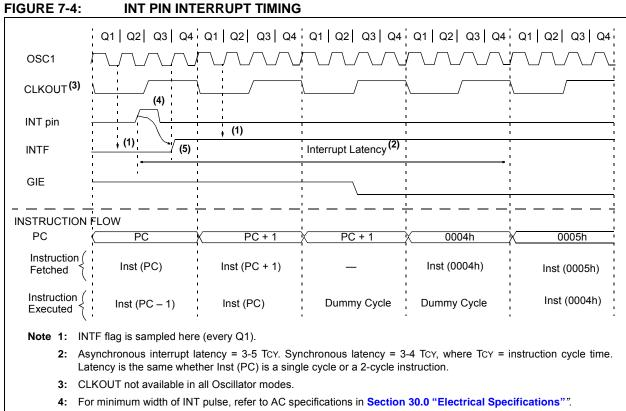
5: INTF is enabled to be set any time during the Q4-Q1 cycles.
