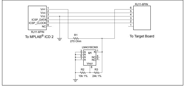
**Note:** The ICD 2 produces a VPP voltage greater than the maximum VPP specification of the PIC16F/LF1946/47.
