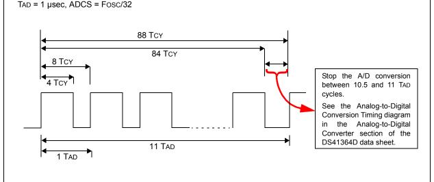
See the ADC Clock Period (TAD) vs. Device Operating Frequencies table, in the Analog-to-Digital Converter section of the DS41364D data sheet.
