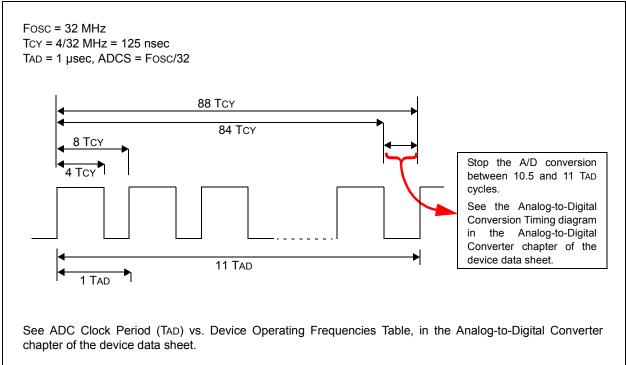
In Figure 1, 88 instruction cycles (TCY) will be required to complete the full conversion. Each TAD cycle consists of 8 TCY periods. A fixed delay is provided to stop the A/D conversion after 86 instruction cycles and terminate the conversion at the correct time as shown in the figure above.
