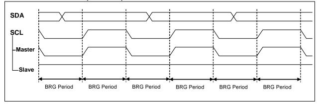
FIGURE 2: EXPECTED OPERATION WITH CLOCK STRETCHING
