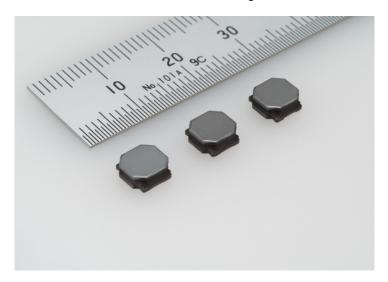
Taiyo Yuden Co., Ltd. has added a new product with height 2.8mm, the NR6028 (6.0x6.0x2.8mm, height is maximum value), to its wire wound power inductor NR60 series lineup used as choke coils in LCD TVs and plasma TVs. This product improves the rated current by about 36% over previous Taiyo Yuden products (inductance 10μH).
