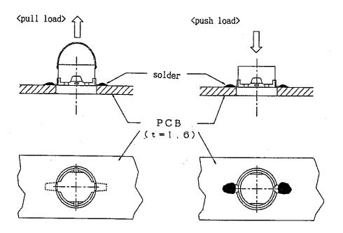
A load shall be applied to inductors soldered on a PCB as above drawing.
