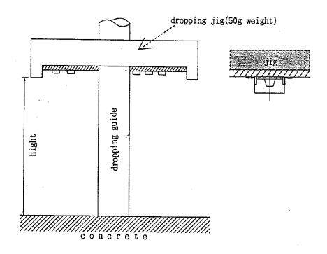
2. TEST METHOD OF EXFOLIATION STRENGTH BETWEEN CORE AND TERMINAL BOARD. (ATTACHED DROWING)
