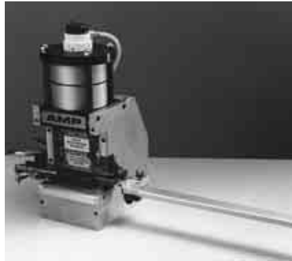
Tube-Fed Ribbon Cable Machine No. 856002-1
