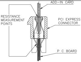
CONTACT RESISTANCE TEST SET UP STRADDLE MOUNT FIGURE 2
