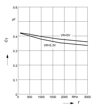
Line capacitance  $C_{T} = f(T_{A})$
