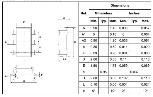
Figure 14. SOT23-6L footprint (dimensions in mm)
