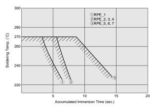
Perform soldering within tolerance range (shaded portion).
