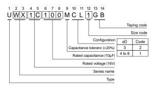
$\bullet$  In the case of size  $\phi 3$  in (  $\,$  ),parentheses, use WX in the 2nd and 3rd digit and put a  $\boxed{2}$  in the 12th digit of type numbering system.
