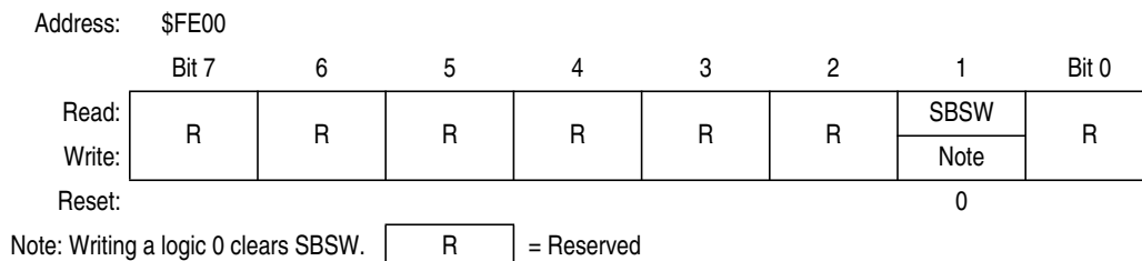
Figure 18-6. SIM Break Status Register (SBSR)
