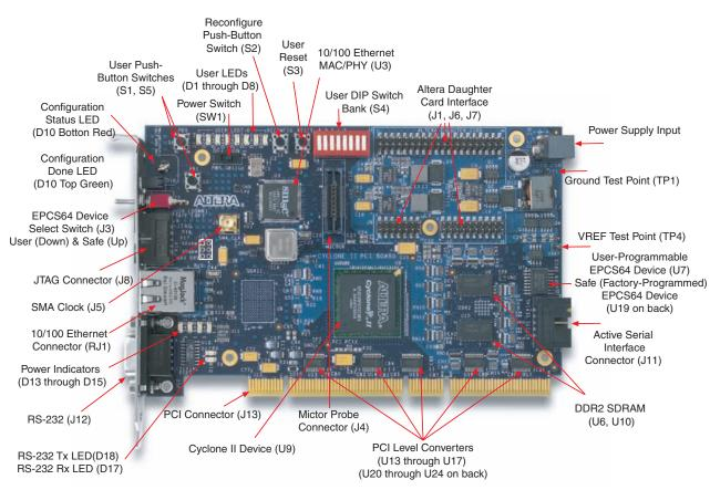
Figure 2–3. Cyclone II EP2C35 PCI Development Board
