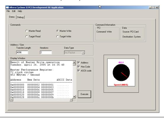
Figure 2-5. PCI Master Write Transaction (Demo Tab)
