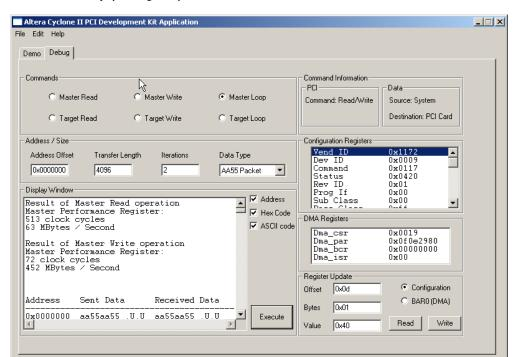
Figure 2-7. PCI Master Loop (Debug Tab)
