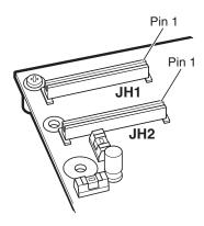
The PMC connector supplies +3.3V, +5V and +/-12V, as required by the PCI specification. However, DC power regulators for these supplies cannot provide enough power to fully satisfy the PCI power specification. The current that the board can supply through JH1 and JH2 is dependent on the design configured in the FPGA. As a general guideline, if the PMC card power requirements exceed the specifications shown in Table 2–14, you must connect an external power source.
