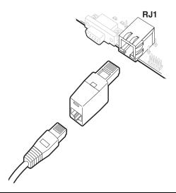
b. Connect the other end of the RJ45 connector directly to the network (Ethernet) port on your host computer.
