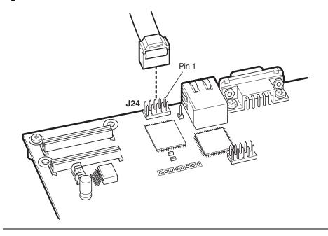
The FPGA's JTAG pins can also be accessed via the Mictor connector (J25). The pins of J24 are connected directly to pins on J25, and care must be taken so that signal contention does not occur between the two connectors.
