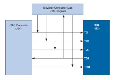
Figure 2–18. JTAG Connector (J24) to Cyclone II Device
