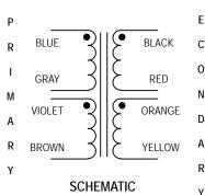
$<sup>^{1}</sup>$  Primary and secondary windings are designed to be connected in series or parallel. Windings are not intended to be used independently.
