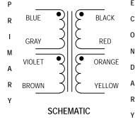
$<sup>^{1}</sup>$  Primary and secondary windings are designed to be connected in series or parallel. Windings are not intended to be used independently.
