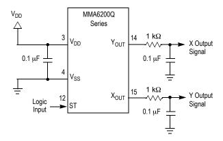
Figure 5. Accelerometer with Recommended Connection Diagram
