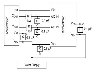
Figure 6. Recommend PCB Layout for Interfacing Accelerometer to Microcontroller
