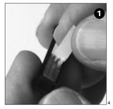
Remove the protective paper lining from the connector cover.
