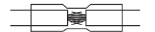
2. Intermingle the wire strands and slide the connector over the joined wires.
