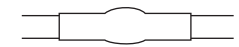
3. Apply heat to the connector until solder and adhesive flows and tubing recovers. Allow the connector to cool.
