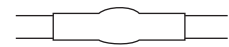
3. Apply heat to the connector until solder and adhesive flows and tubing recovers. Allow the connector to cool.
