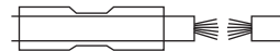
1. Strip wires 3/8" and slide the connector over one of the wires. Separate the wire strands.
