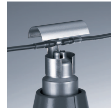
Soldered together and sealed: With the STEINEL solder shrink sleeves, cables can be soldered together and sealed watertight all in one go. Simply fit the solder shrink sleeve over the cable ends, heat up with the hot air tool fitted with the reflector nozzle – done!
