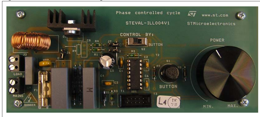
Figure 10. STEVAL-ILL004V1 light dimmer evaluation board
