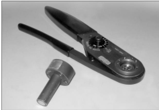
Crimp tooling M317 and locator VGE1 0077A
