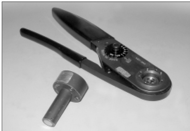
Crimp tooling M317 and locator VGE1 0078A
