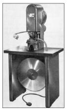
These heavy duty crimping machines are designed for fast and economical production-line crimping of contacts supplied on reels. The machines incorporate the unique DIALMATIC crimp adjustment which permits the machine operator to crimp contacts to wires of different sizes by simply adjusting two knobs.
