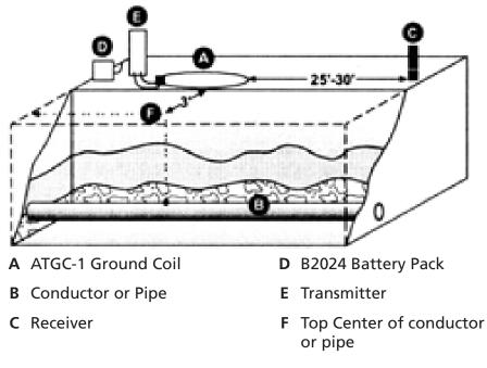
Fig. 2 – Proper distance for initial setup.
