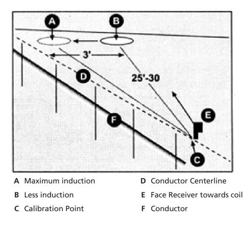
Fig. 4 – Conductor centerline and Coil position adjustment
