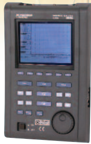
Handheld Spectrum Analyzer with Tracking Generator Model 2652
