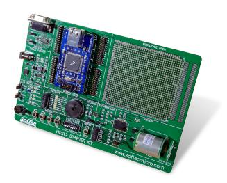
The AK-S12NE64-A Starter Kit is an integrated system designed to provide the user with a complete, ready-to-use embedded Ethernet application. The Starter Kit is built around the Freescale MC9S12NE64 microcontroller, which has a built-in, dedicated Ethernet peripheral. The Starter Kit demonstrates how effectively the MC9S12NE family of microcontrollers can be used in real-world embedded Ethernet applications.
