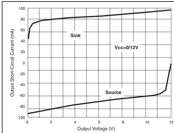
**Figure 2. Output short circuit current vs. output voltage**
