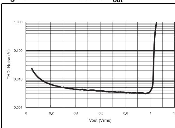
**Figure 12. THD + noise vs.  $V_{out}$**
