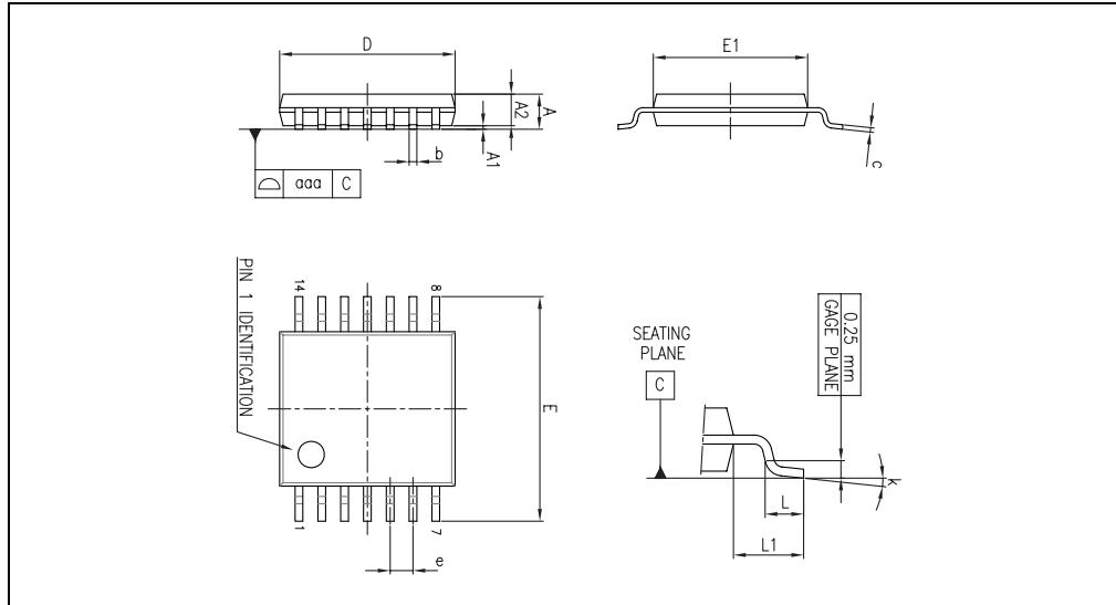
Figure 15. TSSOP14 package mechanical data
