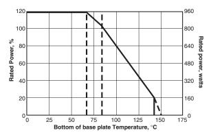
Ohmite's TAP800 Series dissipates 800 watts of power when used with a liquid or air cooled heat sink system. The TAP800 rounds out 600 watt (TAP600) and 1000 watt (TAP1000) product offerings. Applications include variable speed drives, power supplies, robotics, motor control, control devices, and other power designs.
