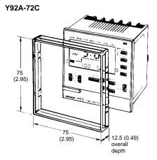
The hard plastic protective cover prevents accidental resetting. It also shields the front panel from dirt and water. The cover is intended for use in areas where unusual service conditions do not exist.
