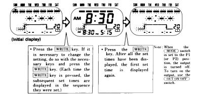
The set times can be checked in the sequence the timer is to operate. In the following example, the times set for today are checked. Set mode selector switch to RUN.
