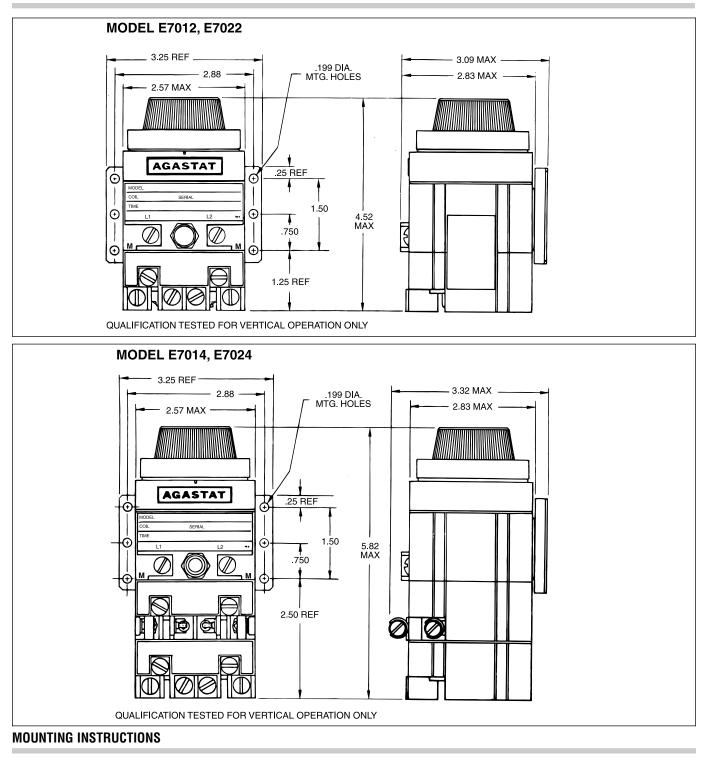
The E7000 Series relay must be mounted in the vertical position. All performance specifications of these units are valid only when they are mounted in this manner. A bracket for mounting the device and the screws and lockwashers required to attach it to the relay are supplied with each unit. Four #8—32 tapped holes are provided in the rear
