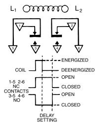
Applying voltage to the coil (for at least .050 second) will instantaneously transfer the switch, breaking the normally closed contacts (1—5 and 2—6), and making the normally open contacts (3—5 and 4—6). Contacts remain in this transferred position as long as the coil is energized. The time delay begins immediately upon deenergization. At the end of the delay period the switch returns to its normal position.
