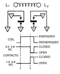
Applying continuous voltage to the coil (L1-L2) starts a time delay lasting for the preset time. During this period the normally closed contacts (3—5 and 4—6) remain closed. At the end of the delay period the normally closed contacts break and the normally open contacts (1—5 and 2—6) make. The contacts remain in this transferred position until the coil is deenergized, at which time the switch instantaneously returns to its original position.
