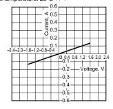
10. Off state leakage current
