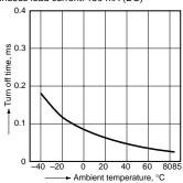
LED operate vs. ambient temperature characteristics
