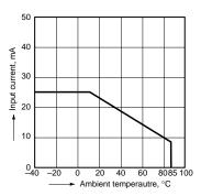
2. Load current vs. ambient temperature characteristics
