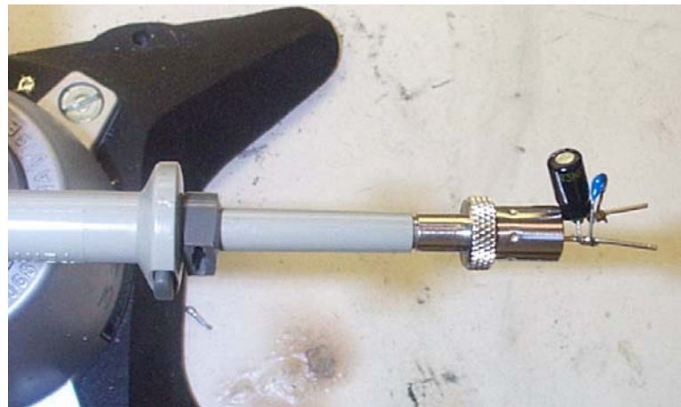
Figure 21 - Oscilloscope Probe with Probe Master 5125BA BNC Adapter (Modified with wires for probe ground for ripple measurement, and two parallel decoupling capacitors added).
