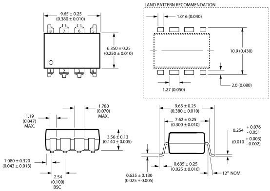
DIMENSIONS IN MILLIMETERS (INCHES). LEAD COPLANARITY = 0.10 mm (0.004 INCHES).
