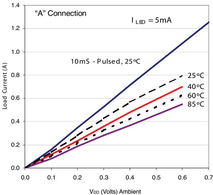
Figure 3. Typical On-Characteristics
