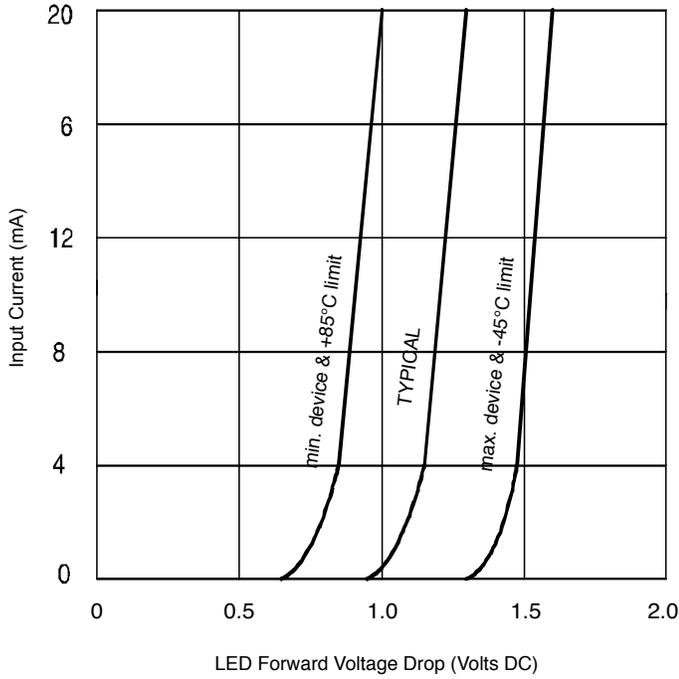
Figure 5. Input Characteristics (Current Controlled)
