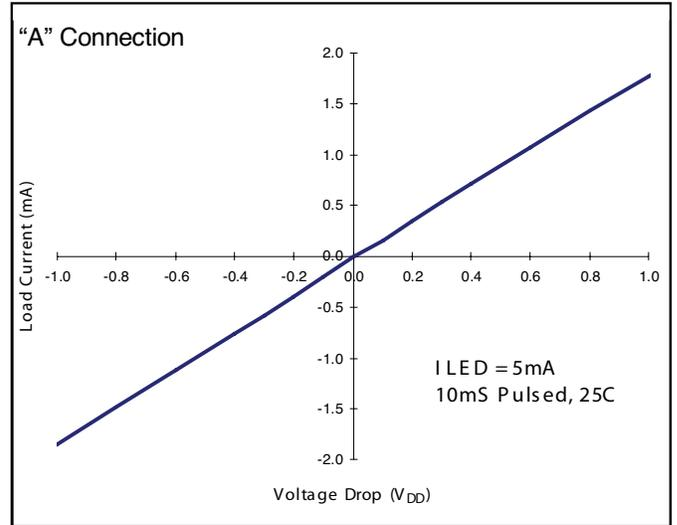
Figure 2. Typical On Characteristics
