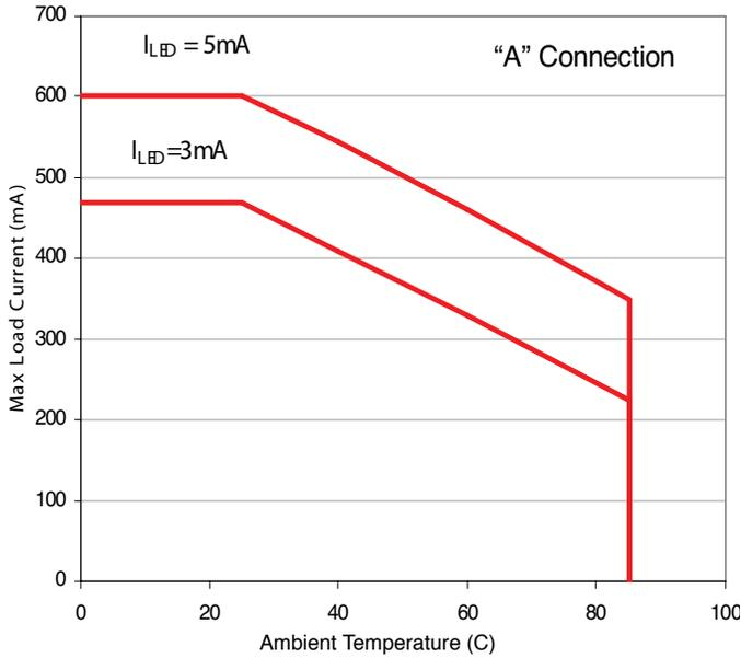
Figure 1. Typical Current Derating Curves
