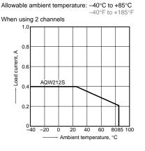
1.-(2) Load current vs. ambient temperature characteristics Allowable ambient temperature: -40°C to +85°C
