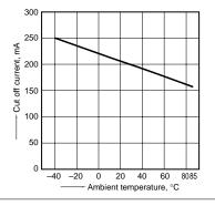
5. LED operate current vs. ambient temperature characteristics Continuous load current: Max.(DC)
