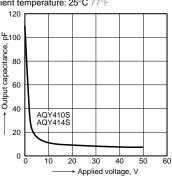
12-(2). Output capacitance vs. applied voltage characteristics
