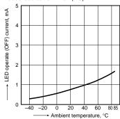
6. LED reverse (ON) current vs. ambient temperature characteristics Sample: All types;
