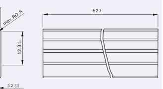
Tube for THT version 25 relays per stick 1'000 relays per box
